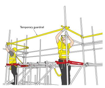
Figure 78: Temporary guardrail to maintain a scaffolders' safe zone for loading bay gate installation and removal. The temporary guardrail is removed once the gate is installed.
