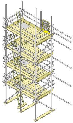
Figure 66: Ladder access bays with single-lift ladders.
