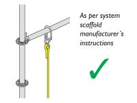
Figure 52: Examples of suitable anchor points and devices.
