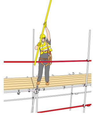
Figure 25: Illustration shows a scaffolder hemping a standard over a guardrail.
