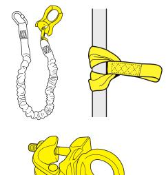
Figure 54: Anchor devices These pictures illustrate the use of connectors specifically developed for use as anchor devices to scaffold standards.
