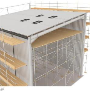
Figure 10: Cross-sections showing examples of collective fall arrest below fragile surfaces, (i) fall arrest safety netting and (ii) birdcage protection deck.
