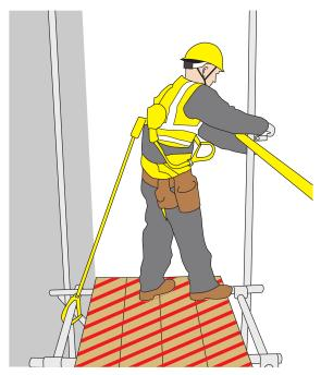
Figure 13: Example of Personal Fall Protection.
