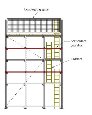
Figure 69: A standalone loading tower with ladder access installed for use by the scaffolders only. Following completion of the loading tower it is highly recommended that the ladders are removed or secured preventing access by others until required for alterations or dismantling.
