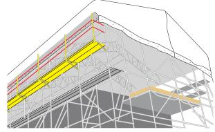
(iii.) Temporary eaves walkways constructed with guardrail protection to allow sheeting operations to be completed from a **scaffolders' safe zone**.
