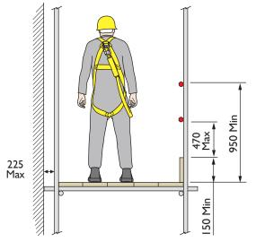
Figure 17: A cross-section of a finished working platform for users
