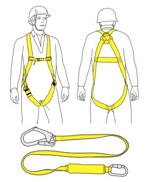
Figure 38: A minimum suggested personal fall protection equipment.
