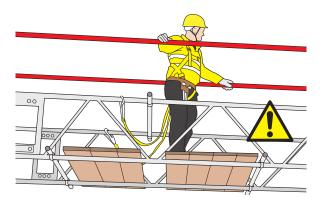
(i) bridging with beams using short transverse temporary boards.
