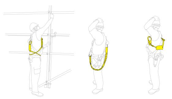
(i). A conventional fixed-length lanyard wrapped around the body and secured when not in use.
