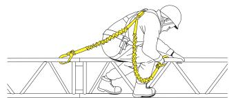
Figure 14: These illustrations show examples of the inherent risk of a fall in scaffolding where personal fall protection equipment will be the primary method of fall protection (e.g. (i) raising and lowering boards and (ii) working without a scaffolders' safe zone).
