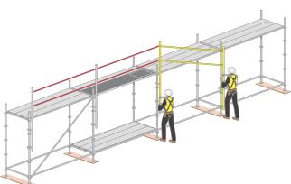
Figure 30: Example of an Advanced Guardrail System (AGS).
