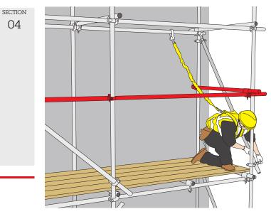
Figure 18: A scaffolder reaching below the single guardrail must be clipped on.
