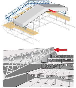
(ii.) Wide gable-end bay scaffolding bay is provided for erecting roof sections from a scaffolders' safe zone. Modular sections are rolled out on special rail and caster systems, to avoid the need for scaffolders to crab the beams.
