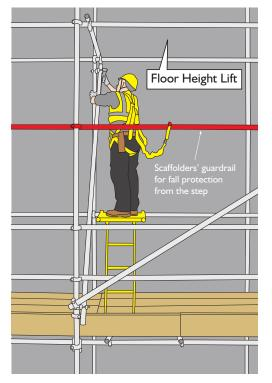
Figure 75: Tall Lifts – Scaffolder using a scaffolders' step to form a floor height lift
