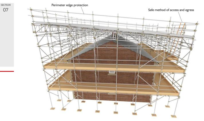
Figure 85: A traditional temporary roof incorporating edge protection and safe access and egress.
