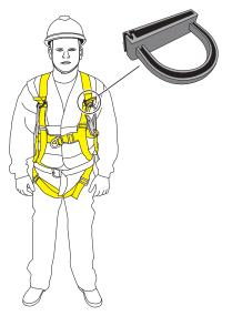
Figure 50: An example of a sacrificial lanyard parking point attached to harness for securing a lanyard when not in use.
