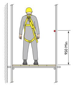
Figure 16: A cross-section of temporary scaffolders working platform to form the minimum scaffolders' safe zone.
