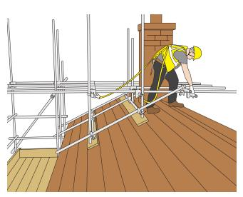
Figure 79: Example of a roof saddle sequence of work with eaves edge protection and continual attachment maintained using a double lanyard system of work.
