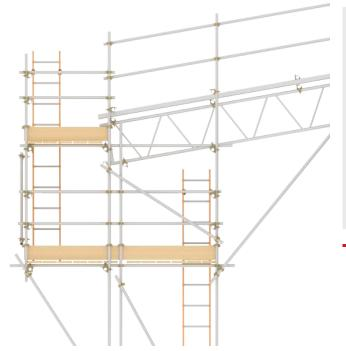
Figure 88: An example of safe access to the roof surface via a cantilevered eaves platform.
