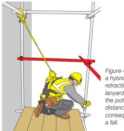
Figure 46: Shows a hybrid selfretracting fall arrest lanyard to minimise the potential fall distance and the consequences in a fall.
