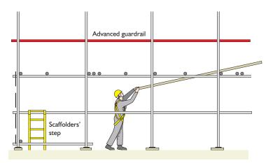
Figure 21: Boarding out the first lift from below.
