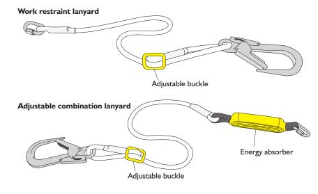
Figure 71: Illustration showing i. a work restraint only that must not be used in fall arrest, and ii. a combination lanyard that can be used in fall restraint and arrest when required.
