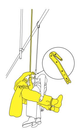
Figure 63: Fully assisted rescue situation. The rescuer has attached the casualty to themself and is cutting the lanyard webbing using a special cutting device that reduces the risk of accidentally cutting the rescue equipment.
