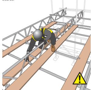
(ii) lacing and bracing beams using longitudinal boards.
