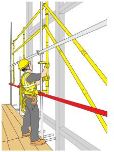
Figure 31: Shows the modified sequence of erection to allow an AGS to be used on the inside face before fixing transoms, ties or inside board brackets above.
