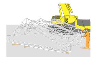
(i.) Modular roof section assembled on the ground and craned into position avoiding the need for scaffolders to crab the beams.
