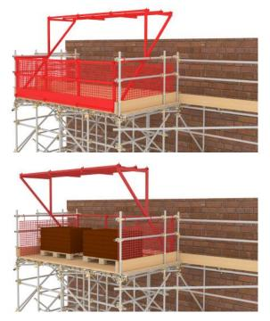
Figure 77: Example of a loading bay gate to maintain collective fall protection for the scaffold users when the loading bay gate is open.
