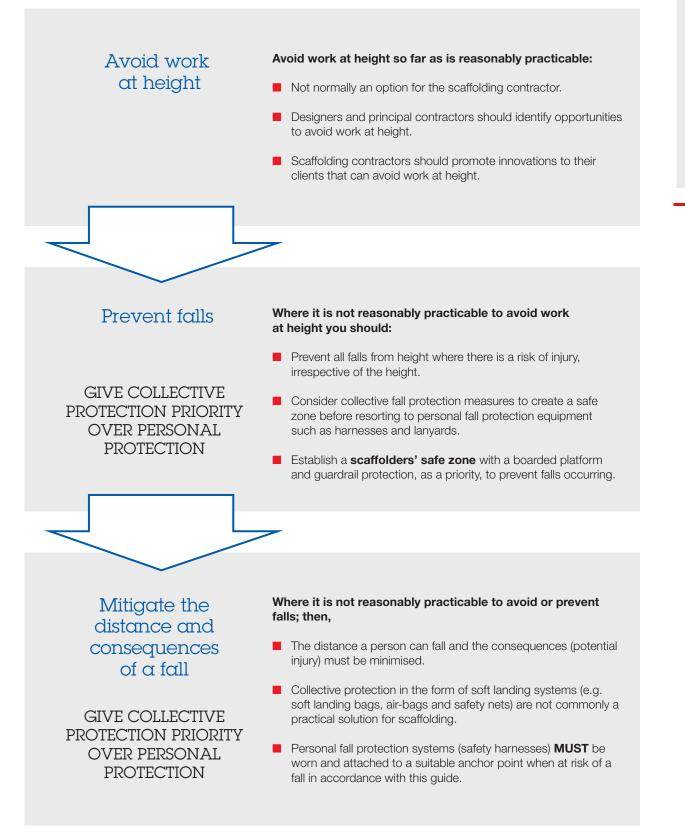
Figure 6: This diagram is a simple illustration of how the 'Work at Height Regulations 2005 Hierarchy of Controls' could be interpreted for scaffolding operations.
