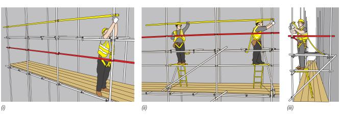
Figure 73: Example of a sequence of work used to erect guardrails in advance for shorter lift heights. (i) Shows the intermediate guardrail installed from the lift below, (ii) a scaffolders' step used to install the main guardrail and (iii) showing the stop-end guardrail. (iv) A 600mm proprietary staging platform being used as an alternative step-up.
