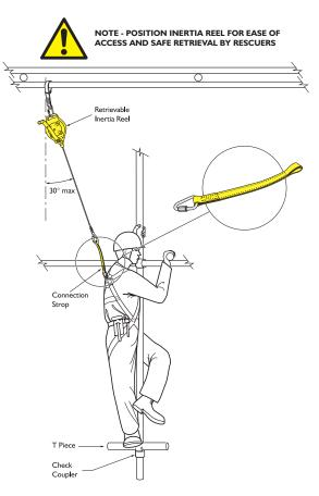
Figure 57: A slung scaffold being erected by a scaffolder utilising an inertia reel as part of the personal fall protection system (inset) Webbing connection strop for use with lines. They provide ease of connection by the scaffolder and emergency release in rescue when using steel lines.
