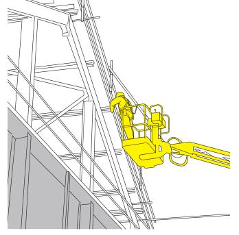
Figure 92: Scaffolder erecting roof edge protection from a MEWP.
