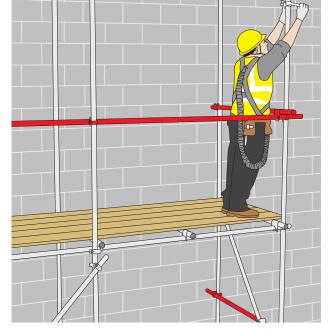
Figure 12: Example of Collective Fall Protection.
