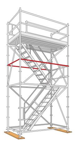
Figure 65: Typical proprietary system scaffold stairway
