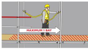
Figure 43: Scaffolder traversing on an unprotected platform remaining attached using a twin lanyard system of work with anchor devices for fixing to standards. The scaffolder should not traverse more than one bay before installing the guardrail that forms the scaffolders' safe zone.
