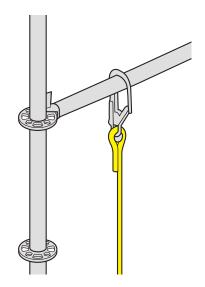
Figure 72: An example of an anchor point for a proprietary scaffolding system as per the manufacturers' instructions.
