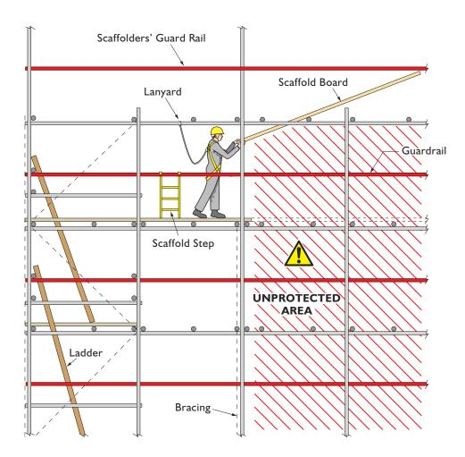
Figure 64: A Scaffolder raising platform boards to the next lift above working progressively backwards towards the ladder access.
