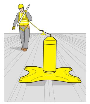
Figure 94: Scaffolder utilising an installed fall protection system for roof access.
